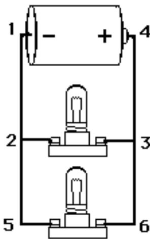
Figure 1. Kelly's Parallel Bulb Circuit.
